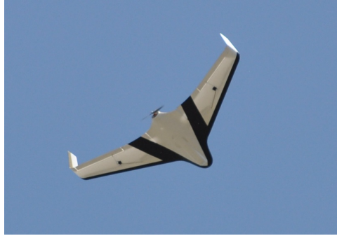
Figure 5.1: Skywalker WiFi-Ferrying UAS.
