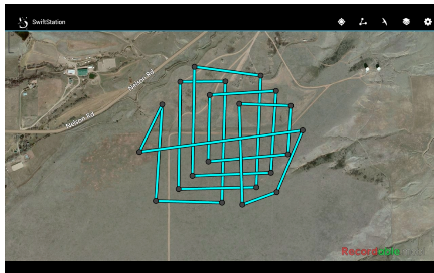
Figure 5.6: Example “Zamboni” Waypoint Path for Throughput Environment Surveys, as viewed through the Black Swift Tech Swiftpilot.
