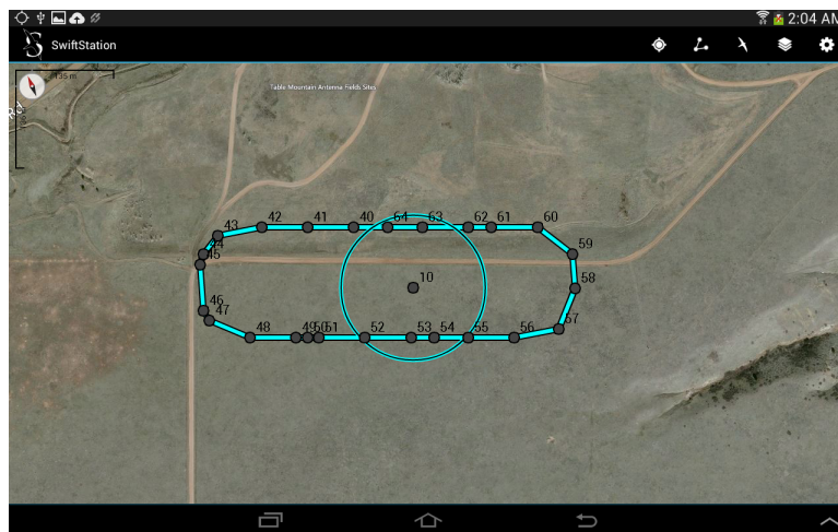
Figure 5.11: Standard ferry “race-track” plan as viewed through the BST tablet interface, with waypoints defined for Knapsack-policy switching.
